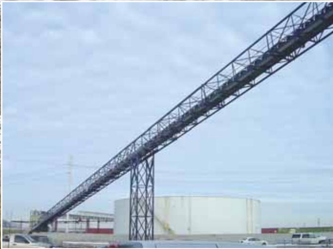
Long-Span and Walk-Through Truss Conveyors.
