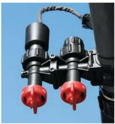
▲ PWM solenoid on the nozzle body instantaneously controls the flow. With the AIM Command option and the Wilger Combo-Rate nozzle bodies, the operator can switch between the AIM Command system and conventional spraying. This gives the operator an option to easily switch between pesticides and spraying larger application rates, such as liquid fertilizer.
