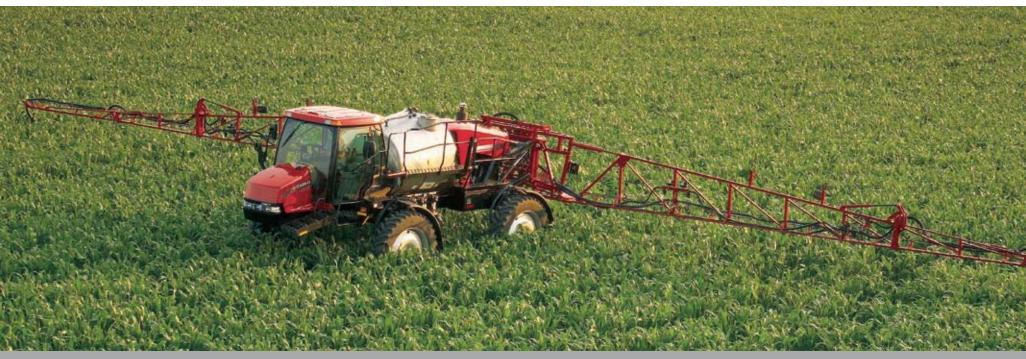
▲ With AIM Command, spraying is done with a constant rate within as much as an **8:1 speed range** through a single nozzle. Also, the application pressure can now be selected and toggled between two preset values without varying that 8:1 speed range.
