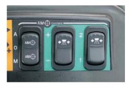
▲ Three conveniently placed switches put true application control right at your fingertips. These switches allow the operator to control the spraying characteristics. The first switch selects between the AIM Command system and conventional spraying. The second switch increases or decreases the pressure setting and the third switch allows the operator to select one of the two preset pressures.
