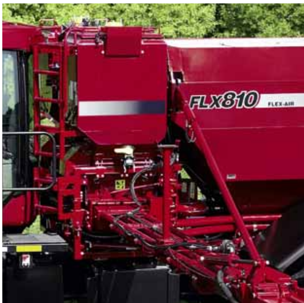
The FLX810 co-ap bins are easy to access and service. Both bins tip out for easy cleaning and extra large doors ease tendering. Both the co-ap bins and the auger housing are lit to help extend your hours of operation.
