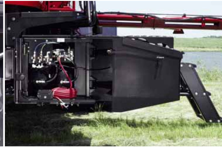
With swing-out compartments on each side, an FLX Series 3-wheel floater allows service access to the air tanks/compressed air and the batteries. It also makes engine service easier. And the storage compartment on the left side is large enough to hold everything from tools to gloves to goggles.
