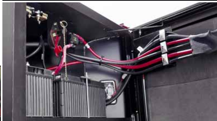
To make battery maintenance a snap, a swing-out compartment that houses the batteries is located on the right-hand side of the 3-wheel chassis. A removable electrical disconnect key can be used to shut down the electrical system for machine maintenance or when the unit is stored for an extended period of time.
