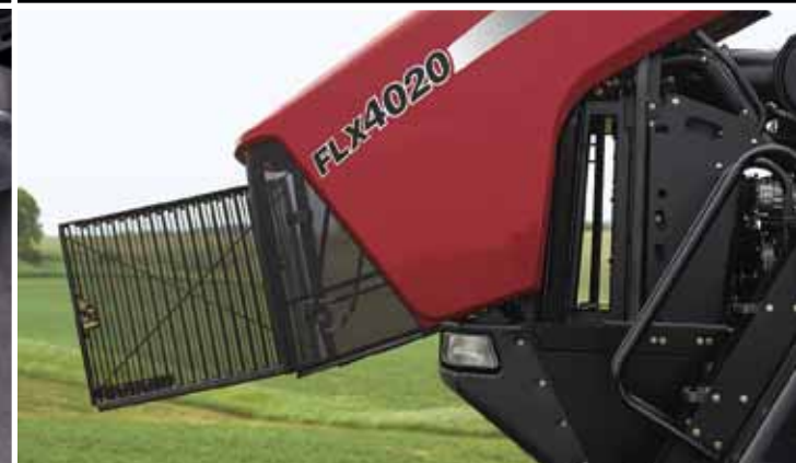
The front-tilt hood of an FLX Series chassis opens easily for access to the engine, coolers and daily checkpoints. The swing-out grille on the FLX4000 Series opens wide to provide hassle-free access to clean the radiator and cooling system.
