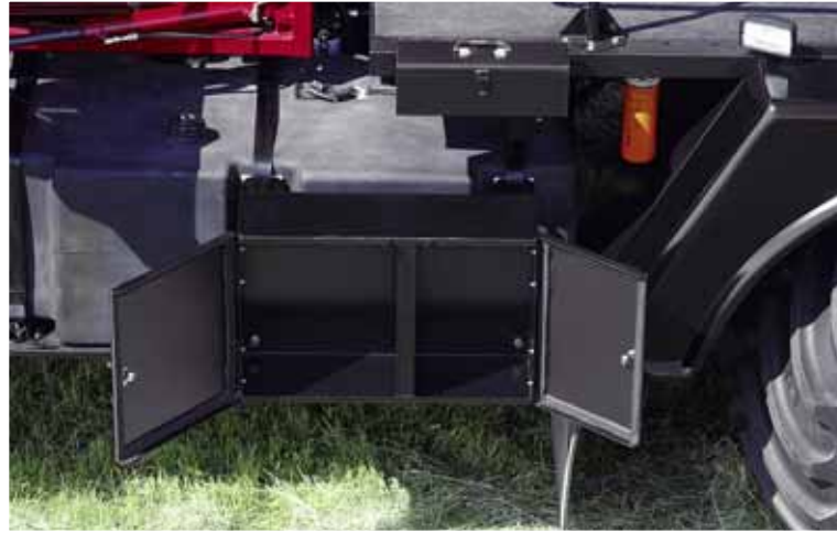
Convenient storage areas are found on both 3- and 4-wheeler chassis (4-wheel chassis shown). A removable toolbox on the 4-wheeler lets you take it to the task instead of running to get a wrench.
